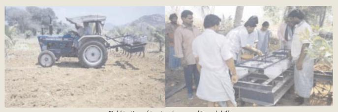
Field testing of tractor drawn multi seed drill
