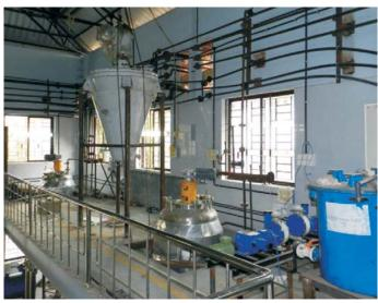
The hydrolysis reactor, nauta mixer & neutralization reactor
