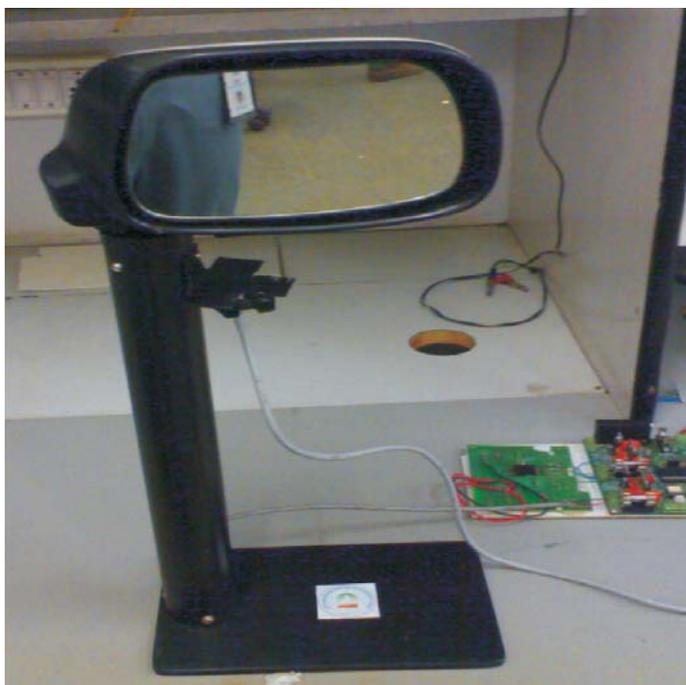
The technology is for automatically adjustable side view mirror for the 4-wheeled automobiles. It aims to provide middle end automobiles with a cost effective option of the automatic side view mirror which can be controlled for horizontal and vertical adjustments from inside the vehicle. Special feature in the mirror includes very near object detection through a sensor and automatic closing of the mirror to prevent mirror damage due to collision while moving on narrow roads with heavy traffic.
