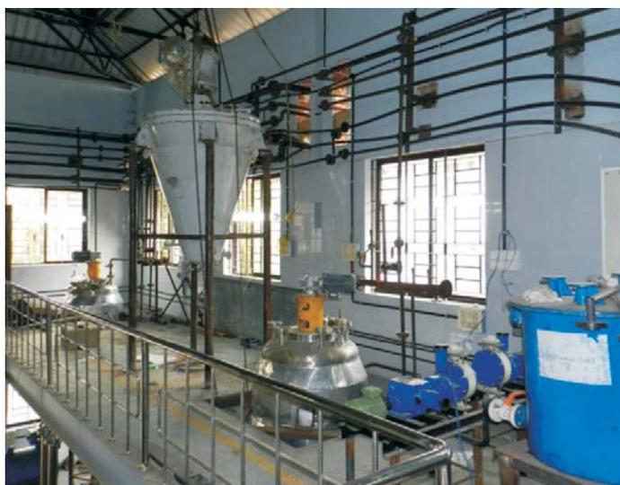
**The hydrolysis reactor, nauta mixer & neutralization reactor**
